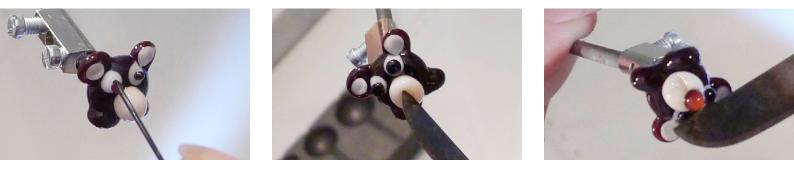
Warm the head thoroughly and then into the oven or vermiculite it goes.
