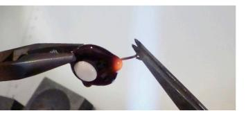
With the tweezers pick up the peg bail, heat the upper end of the body, warm the tip of the peg bail by holding it into the flame for just a second and then stick the tip into the hot soft glass.
