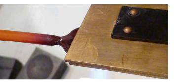
Flatten the blob to a round disc with your pliers, and pull apart both hands while squeezing, to get a thin neck between lolly and rod.
